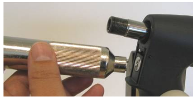
Place special tool in the holes
