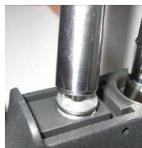
Screw in with special tool
